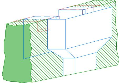
EXTERIOR SCUPPER ISOMETRIC NTS - WITHOUT DIMENSIONS
